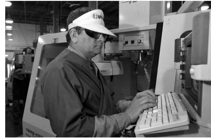
Jim Smith operates a computer numerically controlled milling machine outfitted with a screen-reading speech synthesizer.
